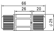
CJ04-1 suitable for 14AWG~16AWG
