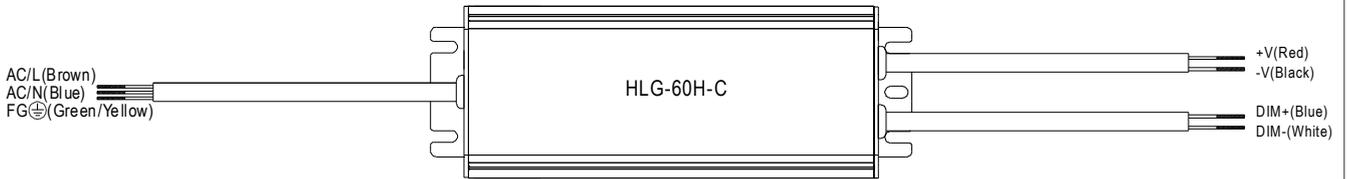
※ Built-in 3 in 1 dimming function, IP67 rated. Output constant current level can be adjusted through output cable by connecting a resistance or 1 ~ 10Vdc or 10V PWM signal between DIM+ and DIM-.
